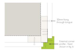
Fig. 8 - External corner detail
