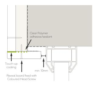
Fig. 12 - Window/door head with Reveal board
