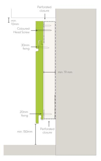
Fig.1 - Top & bottom of cladding detail
