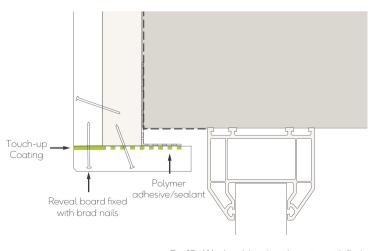
Fig. 17 - Window/door head junction with flush Reveal boards - butt jointed & brad nails
