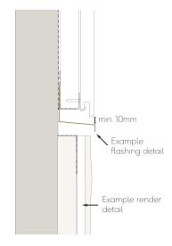
Fig. 23 - Installing cladding above render
