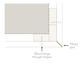
Fig. 10 - External mitred corner detail
