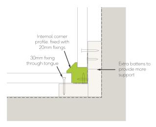
Fig. 7 - Internal corner detail
