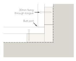
Fig. 9 - Internal butt jointed detail
