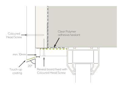
Fig. 15 - Window/door head with angled cut
