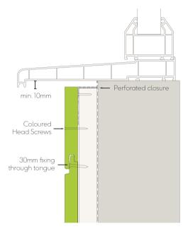
Fig. 3 - Window/door sill detail
