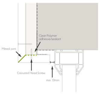
Fig. 14 - Window/door head with mitred joint
