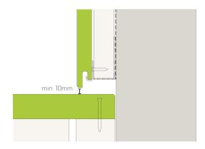
Fig. 5 - Install detail above deck
