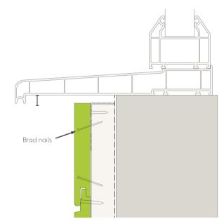
Fig. 16 - Window/door sill junction detail - brad nails
