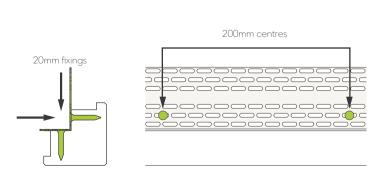
Fig. 6 - Use of perforated closure on corner profiles
