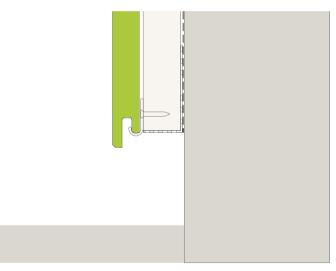
Fig. 19 - First board install
