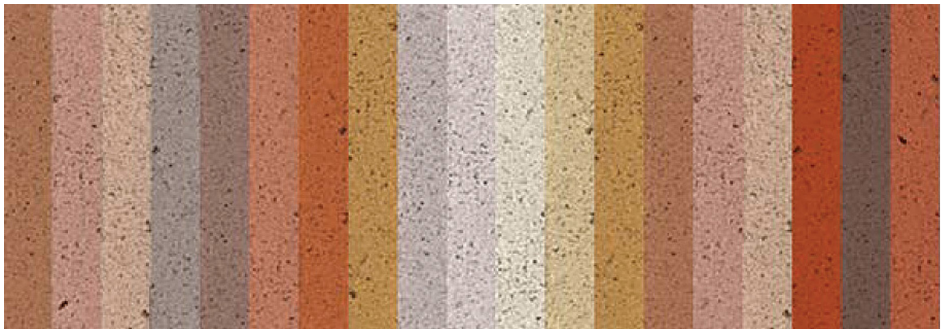
Regulation of the mix proportions is essential to achieve a consistent colour
